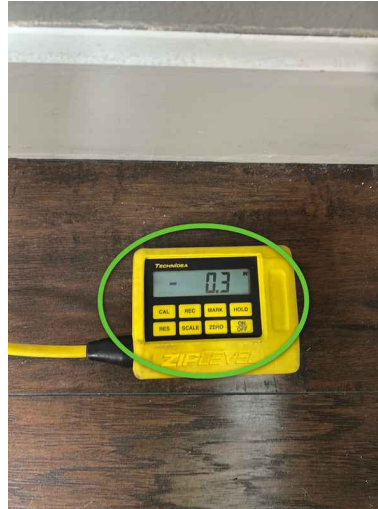
Digital foundation analysis within tolerance
